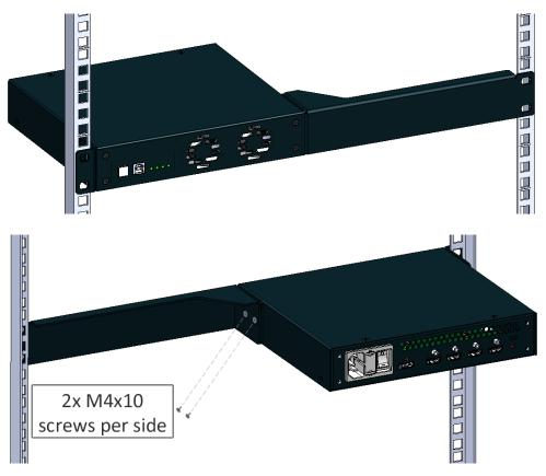
Element of the kit needed: 1x short bracket, 1x long bracket, 4x M4x10 screws.
