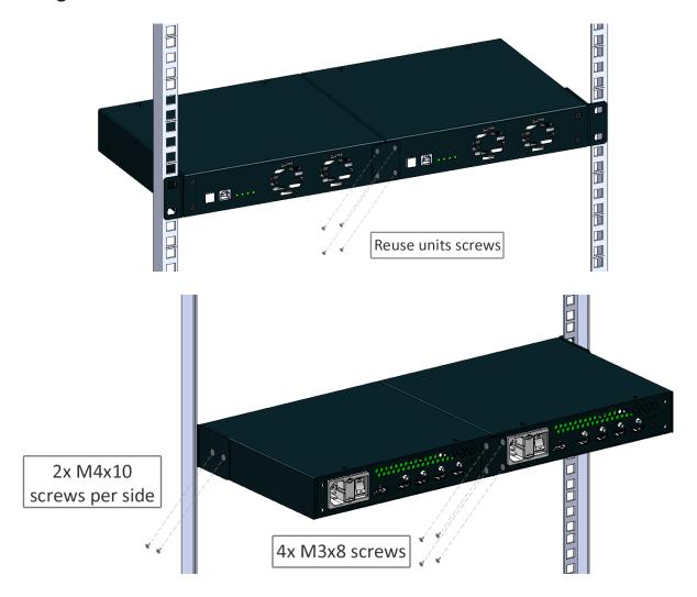
Element of the kits needed: 2x short brackets, 2x pairing plates, 4x M4x10 screws, 4x M3x8 screws.
