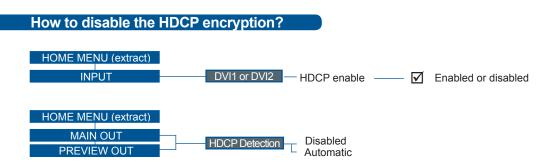
The HDCP Encryption can be disabled on DVI inputs #1 to #2 or/and Main Output / Preview Output. This can be useful when you have a computer which is detecting the HDCP compliance of your switcher and protecting the content by encrypting the signal from this computer. This feature will disable the HDCP compliance on this specific DVI input only.
