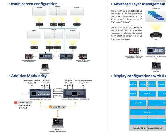
In addition to its four main outputs, LiveCore™ Output Expander 32 - 4K - Ref. LOE032-4K features an independent Dual-Link output for monitoring purposes. This output offers versatile and customizable display options, ensuring effective and flawless show control.
