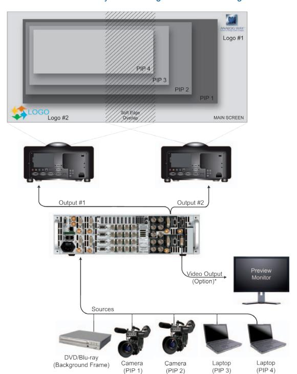
The Di-VentiX II in Embedded Soft Edge mode can seamlessly switch through any of the four available frames stored in its memory.
