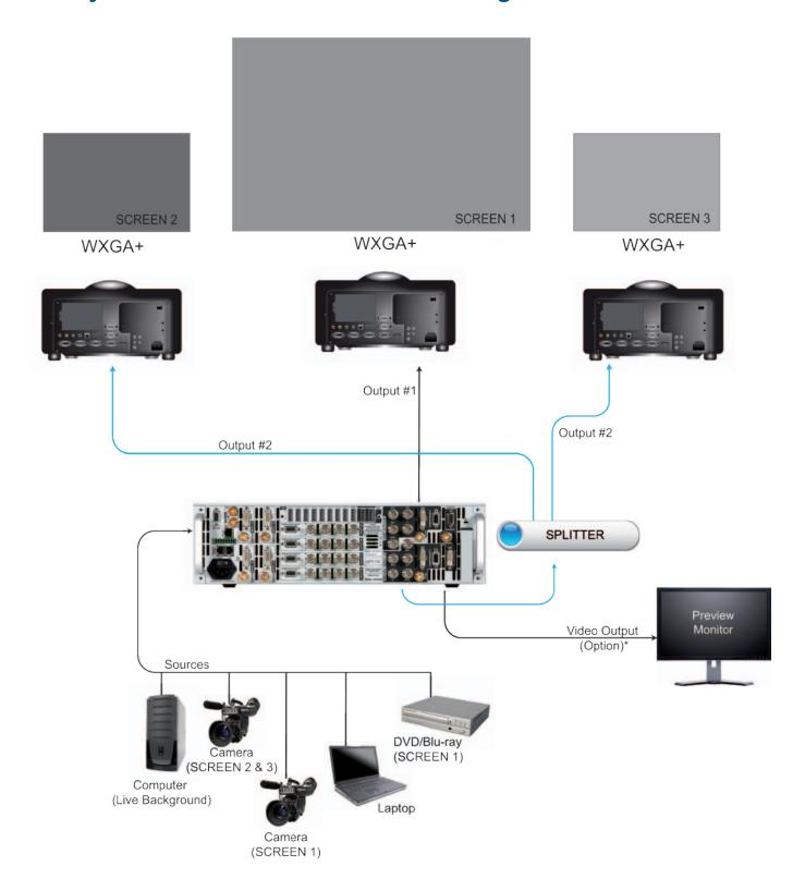
\*Video Output Card (optional) provides SD or HD TV formats in various signals and connectors from Composite Video to HD SDI. This Output can be used to record the show by outputting the same contents as the main output or to display the Preview image on video monitors. In addition, it can be used as a real preview output in case of Sync Matrix or Embedded Edge Blending Mode.
