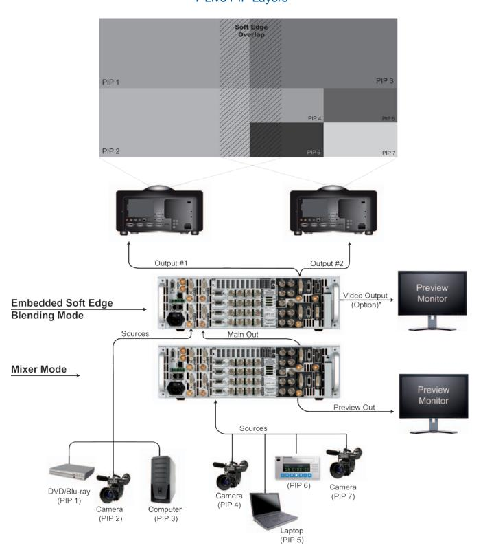
\*Video Output Card (optional) provides SD or HD TV formats in various signals and connectors from Composite Video to HD SDI. This Output can be used to record the show by outputting the same contents as the main output or to display the Preview image on video monitors. In addition, it can be used as a real preview output in case of Sync Matrix or Embedded Edge Blending Mode.
