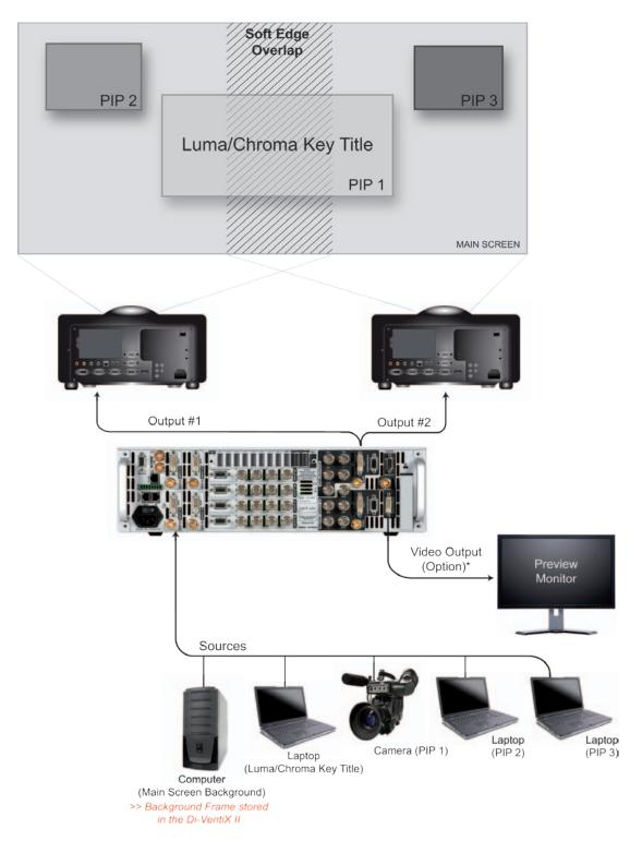
\*Video Output Card (optional) provides SD or HD TV formats in various signals and connectors from Composite Video to HD SDI. This Output can be used to record the show by outputting the same contents as the main output or to display the Preview image on video monitors. In addition, it can be used as a real preview output in case of Sync Matrix or Embedded Edge Blending Mode.
