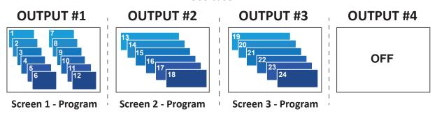
The 6 layers of output #4 can be assigned to another output of the device (on output #1 in this example).
