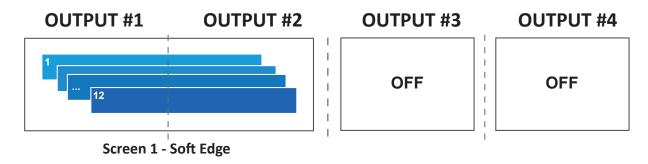
In Soft Edge Blend mode, the active outputs must have the same number of layers. Therefore the additional layers taken from outputs #3 & #4 will be spread to give you 12 total seamless layers of any size or position on your SEB screen.
