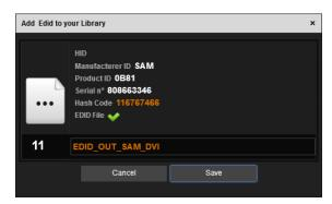
To assign an EDID file from the library to an input plug, just drag and drop it into the selected plug. Please note that you can't drag and drop an EDID file directly from an output plug to an input plug: you must always store the output EDID file into the library first.
